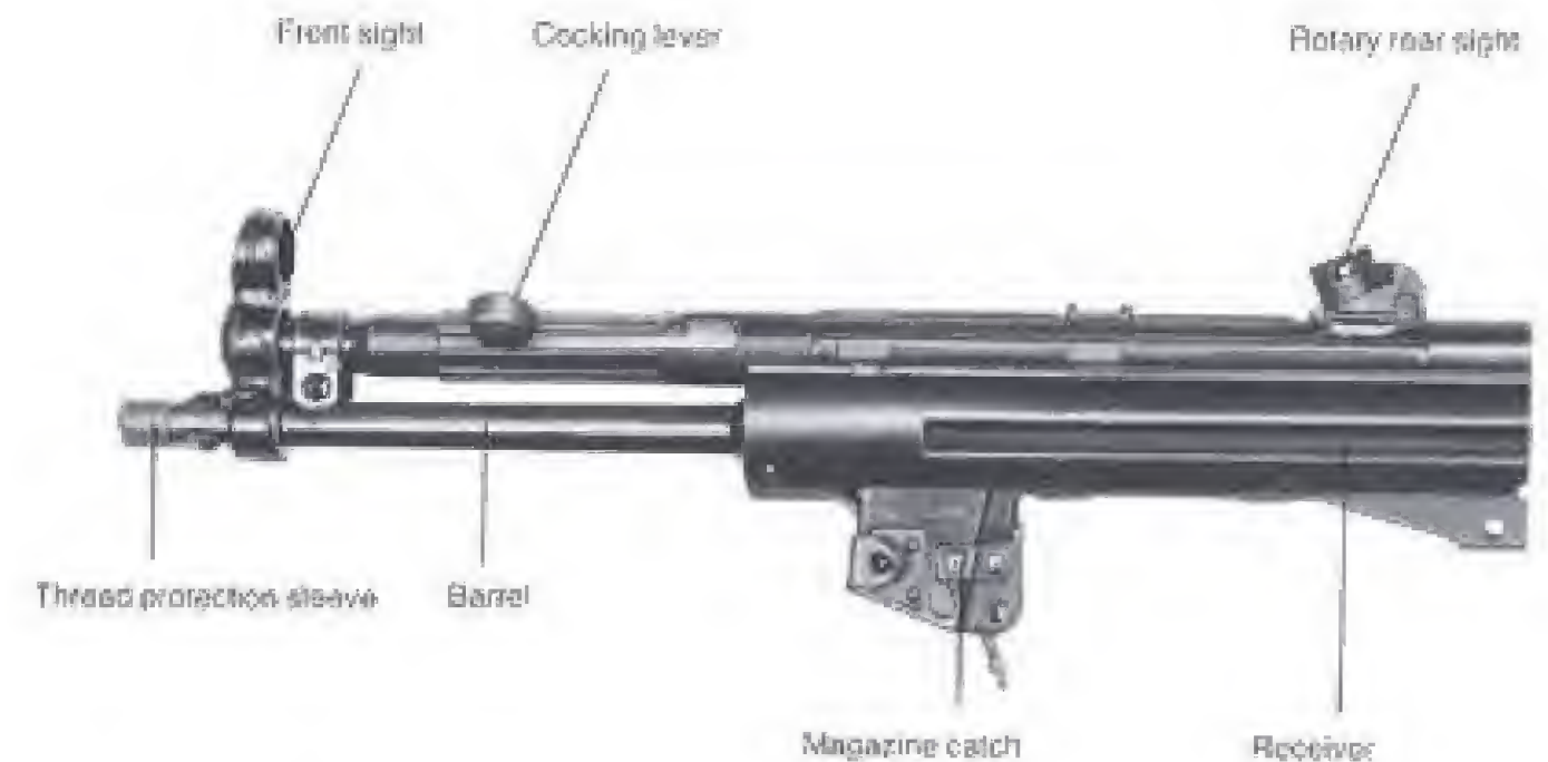
Fig. 4 Receiver with barrel, cocking mechanism and sights
